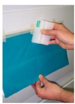
Turn back marking. Keep marking close to substrate without contact. Start application at the middle of the tape hinge. Use a squeegee and firm pressure and apply marking in overlapping strokes from the center to the edges. Work towards your other hand still holding the marking off the substrate. Repeat until liner has been removed completely.
