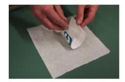
Lay down application tape with non-sticking side on clean flat surface.Drape marking on sticking side starting in the center.
