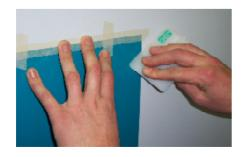
If air entrapments occur peel off marking carefully and retry.
