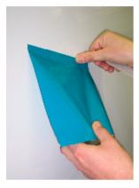
Position marking. Stick one edge of the marking onto the surface without leaving pleats or bubbles. Keep remainder of the marking off the substrate.
